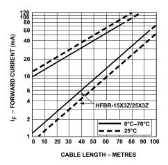
Figure 22: Guaranteed System Performance with Improved Cable
