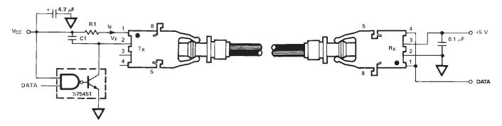
NOTE: The HFBR-25X2Z receiver cannot be overdriven when using the required interface circuit shown in Figure 11.
